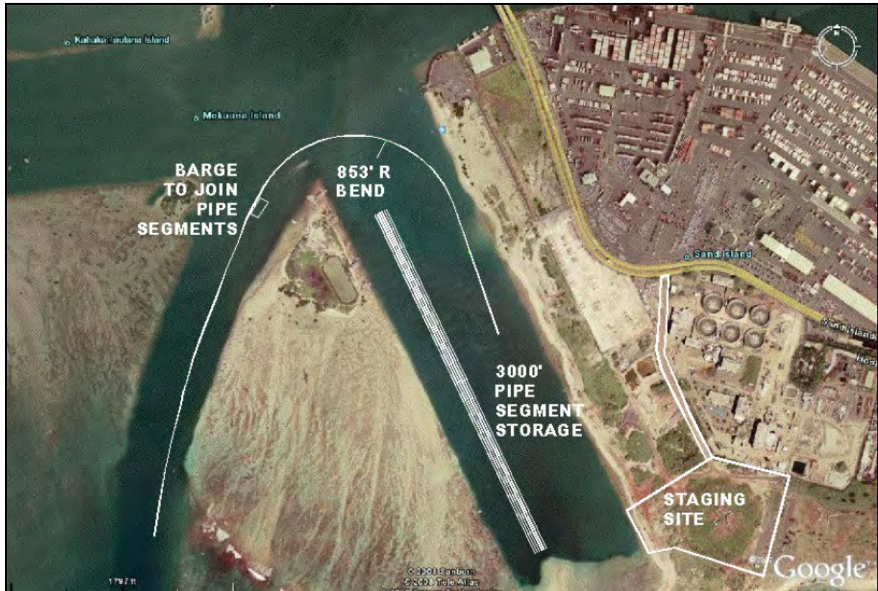
Figure 2-26: Plan for Connecting Pipe Segments and Towing From Ke'ehi Lagoon (Source: Makai Ocean Engineering, Inc.)
