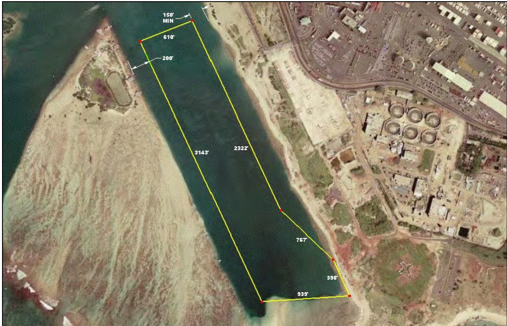
Figure 2-19: Boundaries of Proposed Ke'ehi Lagoon Staging Area (Source: Makai Ocean Engineering Inc.)
