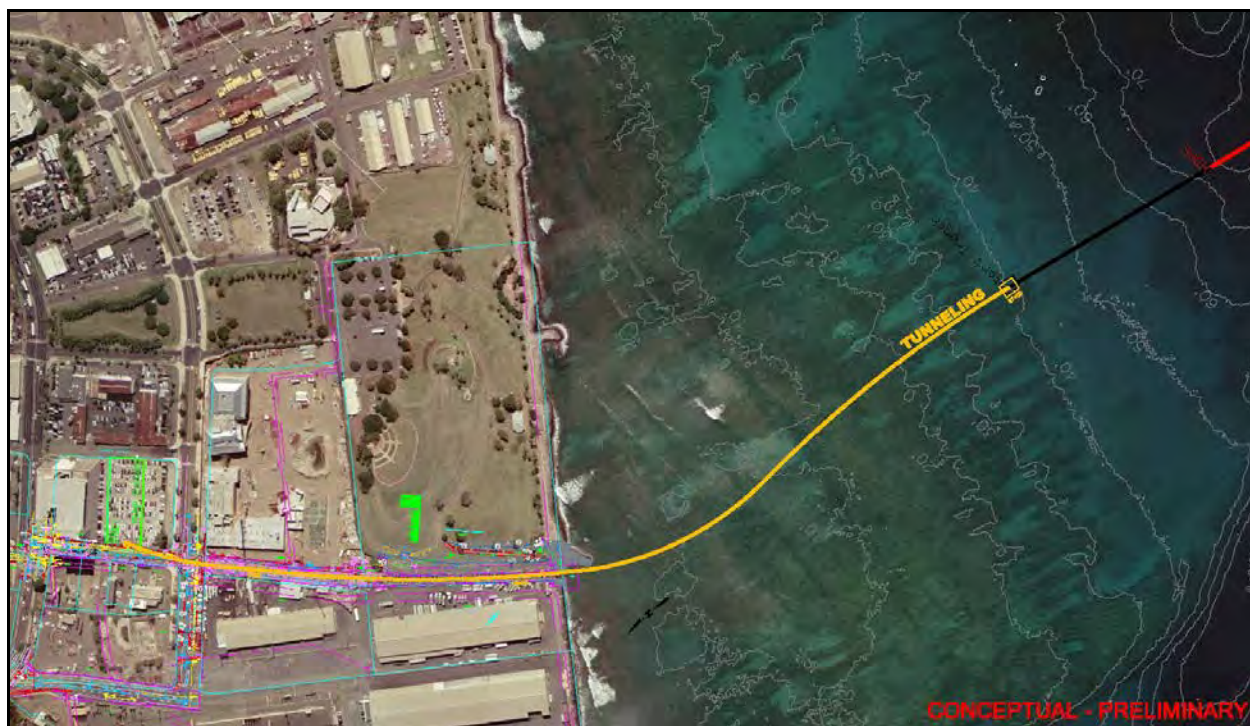
Figure 2-41: Potential Tunneling Route to Breakout Depth
