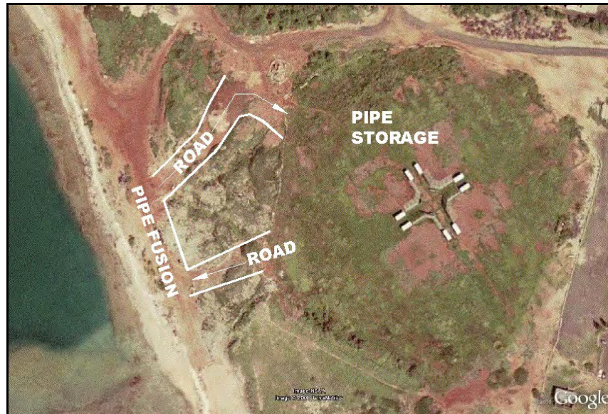
Figure 2-22: Proposed Truck Circulation Routes Within Staging Area (Source: Makai Ocean Engineering, Inc.)
